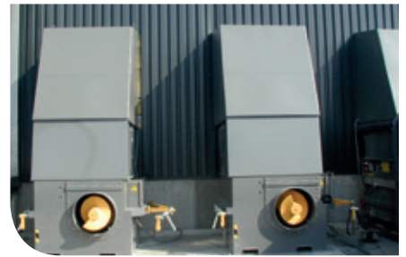
| Screw compactor with centering rails for precise positioning of the container
