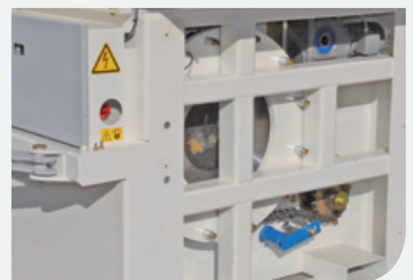
Protected drive unit with labyrinth seal
