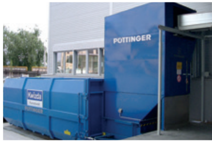
| Screw compactor with centering rails for precise positioning of the container
