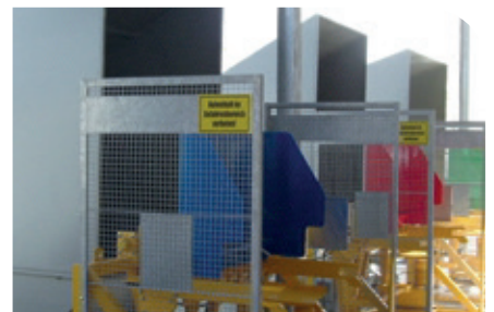
| Tipping device for 660 – 1100 litre containers can be used for any type of installation
