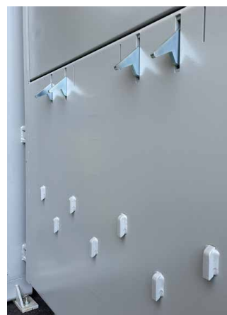
Movable and fixed retaining claws for higher compaction of expanding materials e.g. foils
